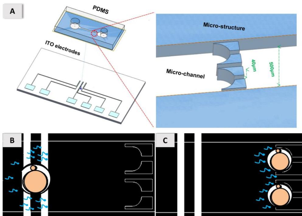
**Figure 1.** Fabrication of the designed DEP microfluidic biochip; (A) actual device of size 5 cm × 3 cm. Bonding of PDMS (microchannel and micro-structures) with the ITO electrode chip. (B) The concept of the experiment is that the mouse oocytes and sperm become trapped on the electrodes for about 1 min with the p-DEP. (C) Co-incubated 1 h in the micro-structures for natural insemination.
