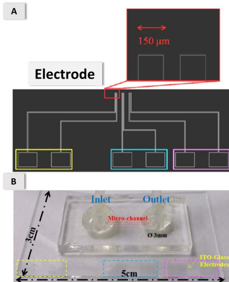
**Figure 2.** (A) Three pairs of parallel linear ITO-glass electrodes. (B) Actual device (5 cm  $\times$  3 cm). Each gap between the electrodes has width 100  $\mu\text{m}$ ; each electrode has width 150  $\mu\text{m}$ .
