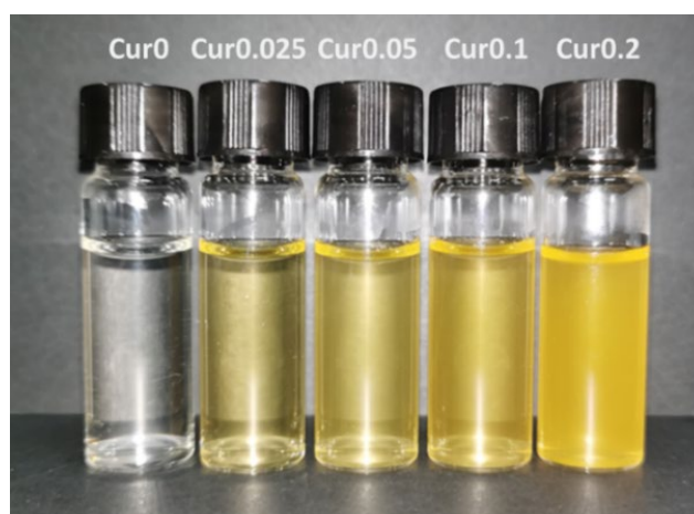
Figure 1. Film-forming solutions (FFSs) with different concentrations of Cur (prepared with a 4:6 mixture of GEL and CS).
