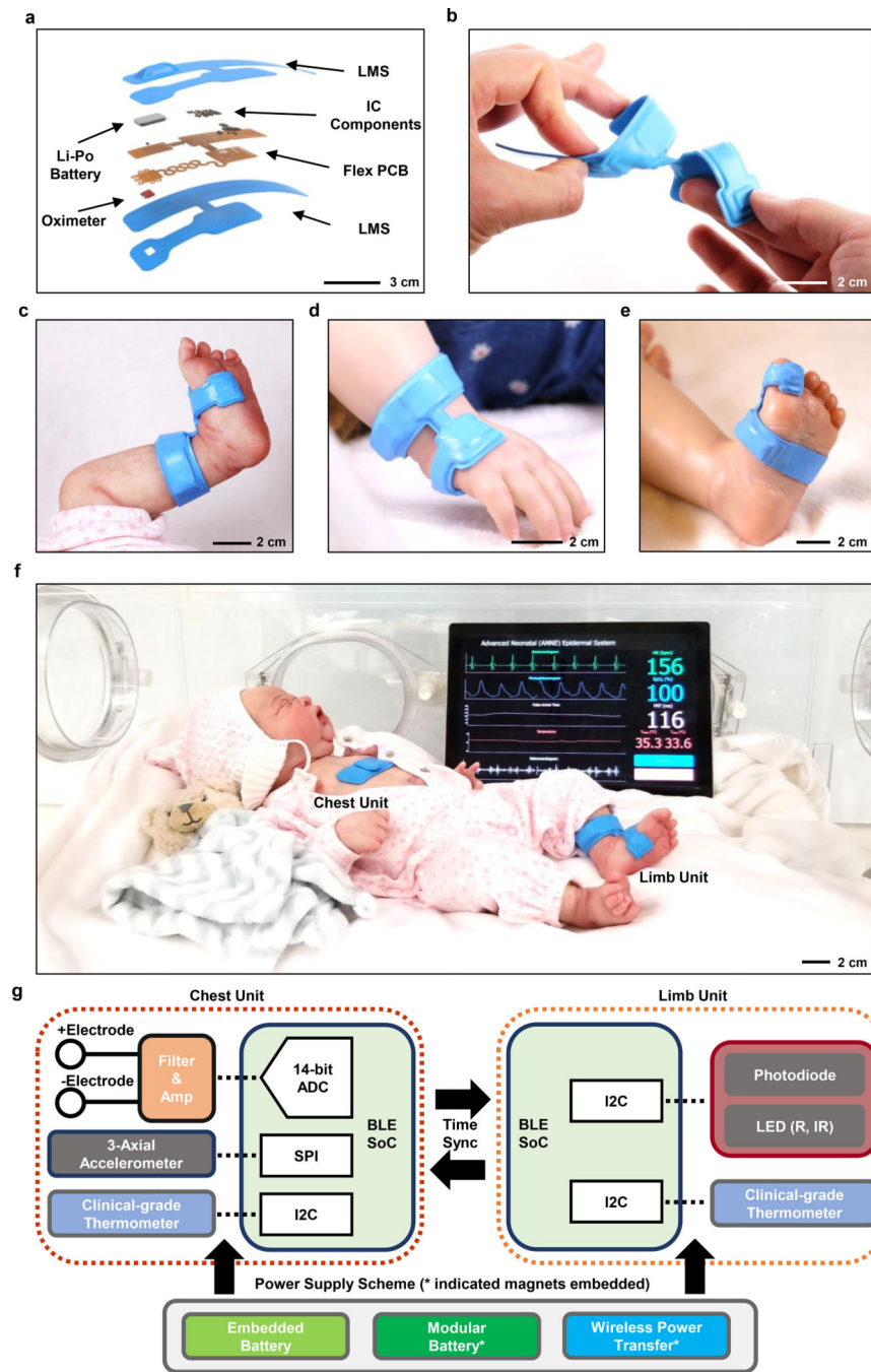
Fig. 2. Designs and photographs of a wireless limb unit for physiological monitoring of neonatal and pediatric patients and block diagram of the system operation.
