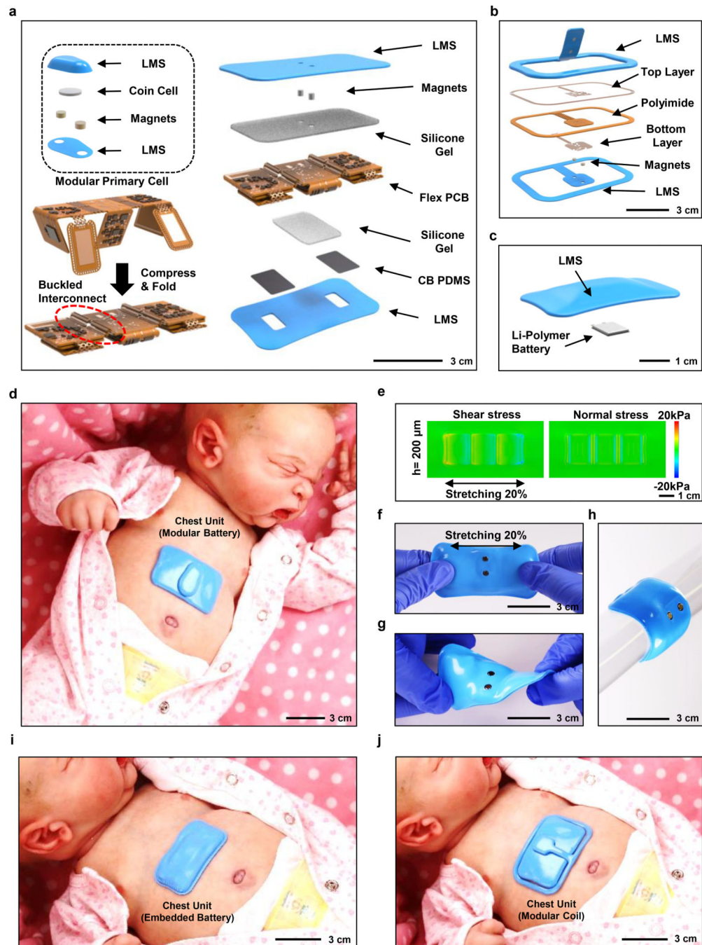
Fig. 1. Designs, mechanical characterization results and photographs of a soft, wireless chest unit for physiological monitoring of neonatal and pediatric patients.
