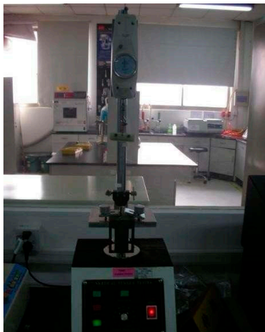
Figure 19. WDW-100 tensile shear strength device.
