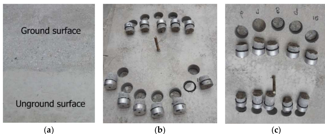
Figure 11. Pull-off test: (a) surface conditions before TRC strengthening; (b) failure mechanism with unground surface; and (c) failure mechanism with ground surface.
