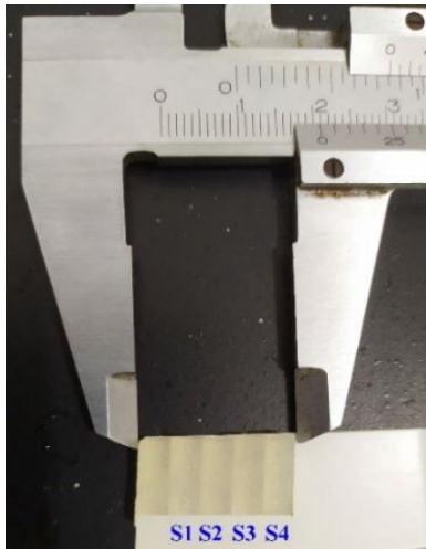
Figure 2 Samples with varying agar concentration values s_1 to s_4 (low to high concentration), and similar cross sections.
