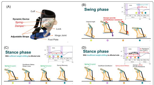
**Fig. 1** Schematic diagram of the device, including the **a** structure and **b** dynamic components providing plantarflexion resistance in the swing phase, **c** dynamic components restored on the stance phase with sufficient weight shifting to the affected side, and **d** dynamic components not restored in the stance phase with insufficient weight shifting to the affected side
