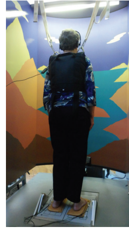
FIGURE 2: NeuroCom EquiTest system. Participants stood on customized soles with embedded vibrating units during all trials.
