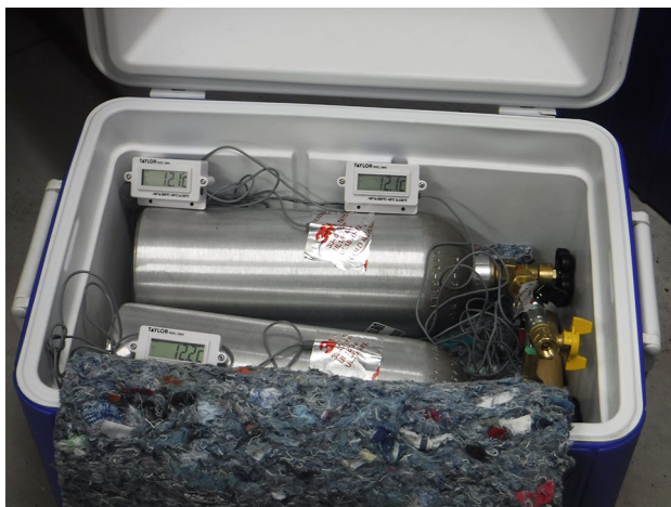
Figure 2. The full experimental apparatus, with two CO 2 cylinders connected by the manifold (Fig. 1), inside the insulated chest, with the three thermocouples attached.
