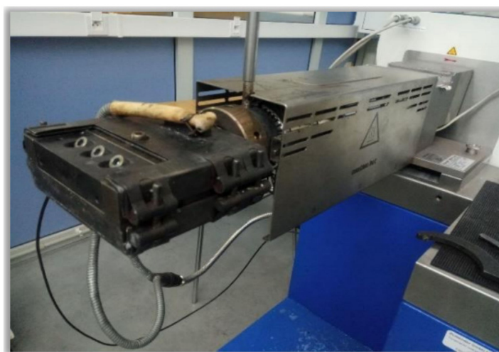
Figure 4. The single-screw extruder (Brabender ® , Duisburg, Germany), equipped with a narrow slot head (photo taken by authors of manuscript, Lukasiwicz Research Network, Poland, 2018).
