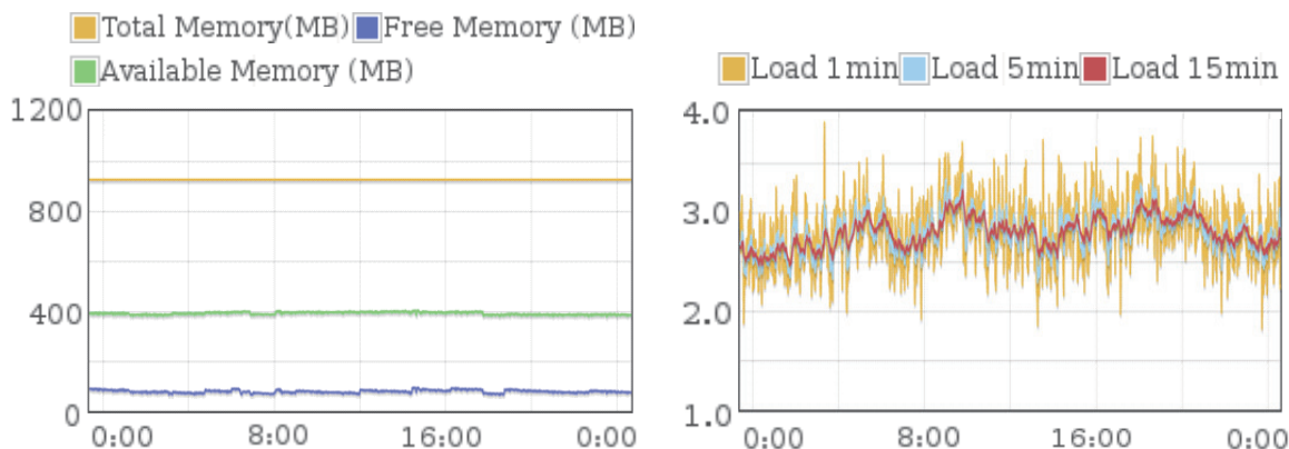
Figure 7. Usage status of system memory and CPU that collecting feature data using a Raspberry Pi.
