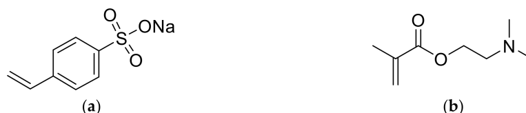
Figure 1. Chemical structure of (a) NaSS anionic monomer and (b) DMAEMA cationic monomer.
