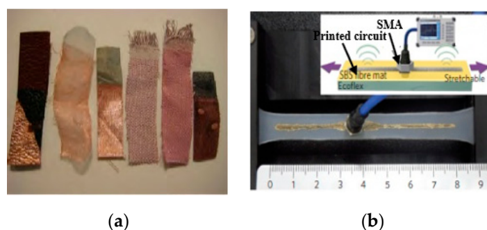
Figure 1. (a) Different conductive textile material [96], (b) conductive composite materials [135].
