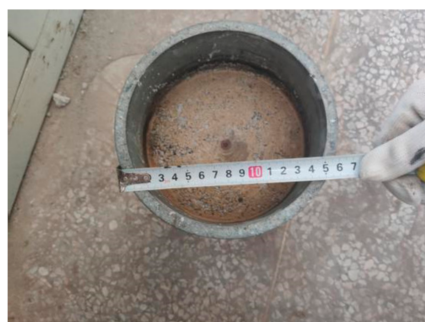
Figure 5. Crushed stone mixture specimen after preparation.
