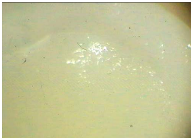
Figure 3: Combined (adhesive and cohesive) failure
