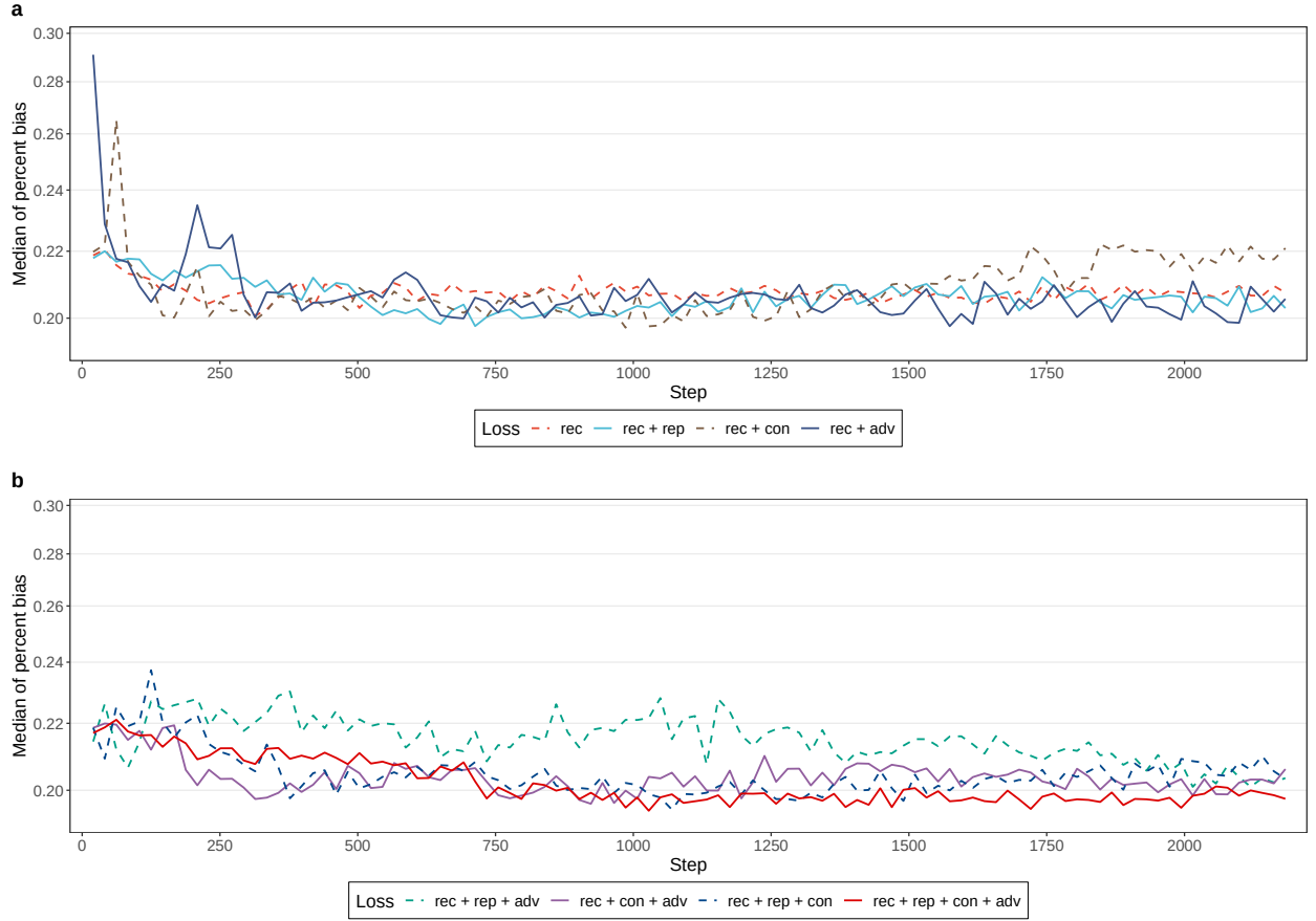
Supplementary Figure 15 The ablation test evaluates the contribution of four losses: reconstructive loss (rec), representation loss (rep), contrastive loss (con), and adversarial loss (adv). Grid search strategy is used to determine the optimal weights for different losses, and the median percent bias computed from the validation set is used to quantify the performance. The network layers are consistent during the evaluation. The plot shows the performance of reconstruction loss combined with (a) a single loss and (b) multiple losses, using the optimal weight of each loss. The weight for rec is fixed at 1, and the weights for the other losses vary across 0.01, 0.05, 0.1, 0.5, and 1. The optimal weights for different losses in each combination are: rec + rep ( w_{rep}=0.01 ), rec + con ( w_{con}=0.01 ), rec + adv ( w_{adv}=0.5 ), rec + rep ( w_{rep}=0.01 ) + adv ( w_{adv}=1 ), rec + con ( w_{con}=0.01 ) + adv ( w_{adv}=1 ), rec + rep ( w_{rep}=0.5 ) + con ( w_{con}=0.01 ), rec + rep ( w_{rep}=0.1 ) + con ( w_{con}=0.1 ) + adv ( w_{adv}=1 ). Source data are provided as a Source Data file.
