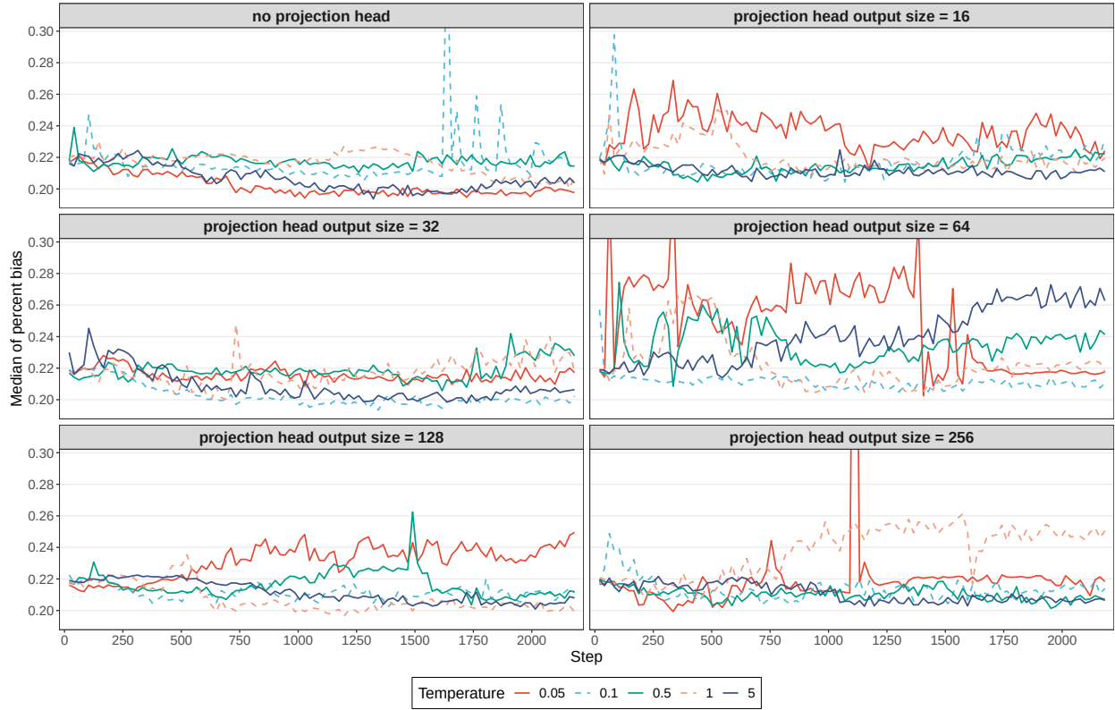
Supplementary Figure 17 Based on the hyperparameters determined in the previous experiments, we further fine-tuned the projection head and temperature used in our contrastive loss. We use grid search to evaluate the performance of LEOPARD without a projection head and with a projection head of different output sizes. The temperature varies across 0.05, 0.1, 0.5, 1, 5, 10, and 30. Based on our experiments, LEOPARD is trained with a temperature of 0.05 without using a projection head. Source data are provided as a Source Data file.
