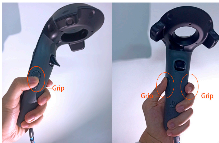
Figure 5. Using the grip key of the HTC Vive handle as the climbing grip key.
