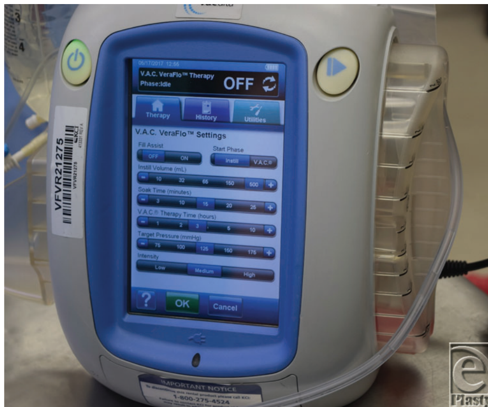
Figure 6. The VAC Veraflo suction device display showing the settings for instillation as well as negative pressure wound therapy. Fill Assist is turned “OFF” and the Start Phase reads “Instill”. The Instill Volume (mL) reads 500 for the amount to be instilled into the abdomen and the “Soak Time (minutes)” is set at “15 minutes.” VAC Therapy Time (hours) is reading set at “3.” The Target Pressure (mmHg) reads “125” and Intensity is read at “Medium.” The side canister is currently a 500 mL container but was increased to the larger capacity container of 1000 ml.
