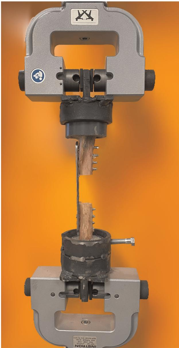
**FIGURE 2** The locking plate construct within the testing frame. The specimen was placed within the custom-made steel grips which allowed for a stable fixation within the mechanical testing frame. The screw in the bottom grip was tightened before the construct testing to prevent the rotation of the specimen during testing [Color figure can be viewed at [wileyonlinelibrary.com](http://wileyonlinelibrary.com)]
