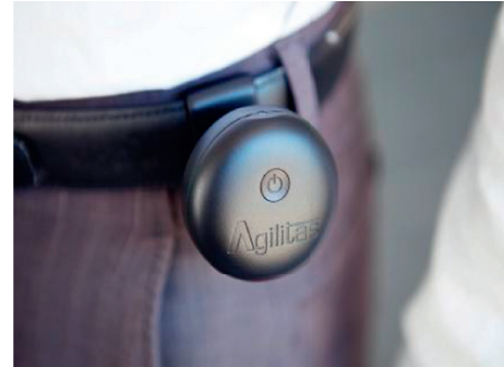
FIGURE 2: The belt-worn freeze-detecting visual cueing device. Note: the image shows the pilot light pointing upwards. By turning the device, the orientation of the visual cue can be personalised for each individual.
