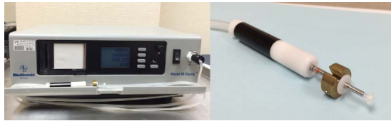
FIGURE 1. Pneumatometer and its probe, which has a flat tip with an external diameter of 5.3 mm. The weight on the probe is used only for tonography.
