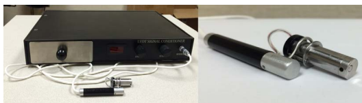
FIGURE 4. Custom digital Schiøtz tonographer and its probe, which has a plunger with a concave tip and an external diameter of 10 mm.
