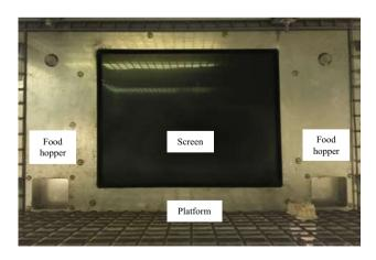
Fig. 1 Touch screen set up for squirrels. The screen is at the centre with two food hoppers, one on each side. Stimuli are presented at the eye level of squirrels and correct stimulus leads to food delivery on the corresponding side
