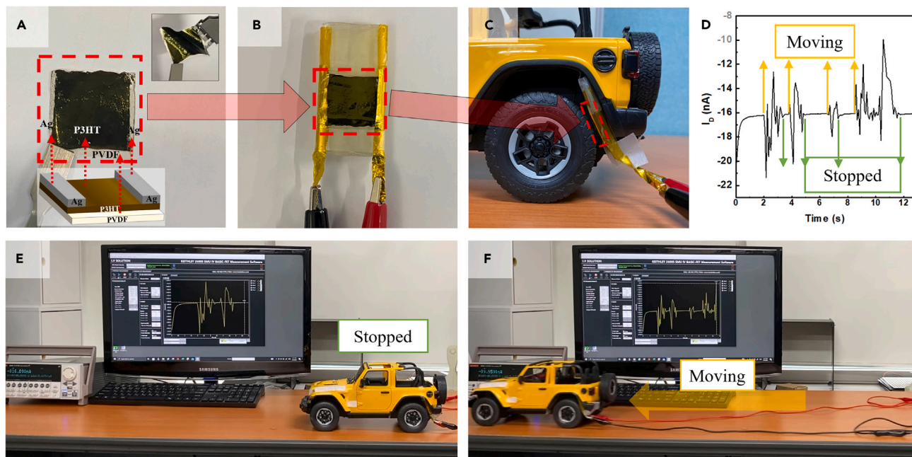
Figure 9. Procedure for validating the feasibility of using the current amplified from a tire of an RC car
