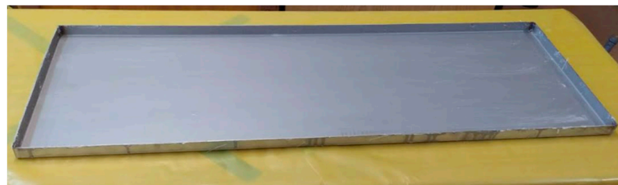
Figure 1. Mold for production of composite sample.
