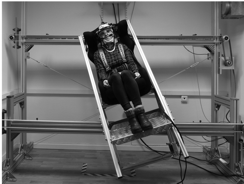
FIGURE 3. Picture demonstrating passive whole-body movement during vestibular stimulation. Subject is positioned in a dark room without visual information and is wearing an eye tracker (Chronos C-ETD) for recording of the VOR response due to the head tilt. Extrication collar and hook-and-loop straps stabilized the movement as to obtain an isolated and stable vestibular activation through relieving neck muscles and minimizing proprioceptive input. Reprinted from Wibble T, Pansell T. Vestibular eye movements are heavily impacted by visual motion and are sensitive to changes in visual intensities. Invest Ophthalmol Vis Sci. 2019;60:1021–1027. © 2019 The Authors. Published by the Association for Research in Vision and Ophthalmology (ARVO).
