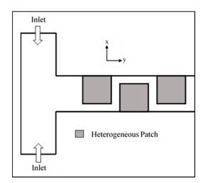
**Figure 15.** Schematic diagram of the new micromixer design with spacing between adjacent charged patches.
