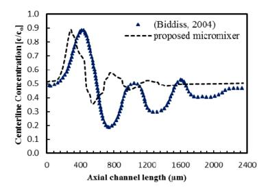
**Figure 18.** Comparison of normalized concentration distributions at centerline along the channel length between the proposed micromixer and the micromixer reported by Biddiss [8] at E = 280 V/cm.
