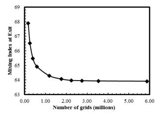
Figure 4. Grid-dependency test for the mixing index at the exit.
