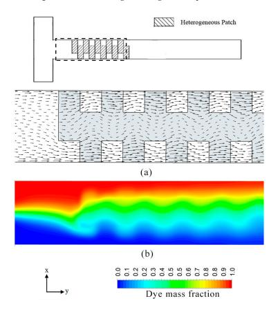
**Figure 2.** Mixing in the reference micromixer on *x-y* plane at E = 400 V/cm: (a) velocity vectors at  $z/H_c = 0.33$  and (b) dye mass fraction distribution at  $z/H_c = 0.5$ .
