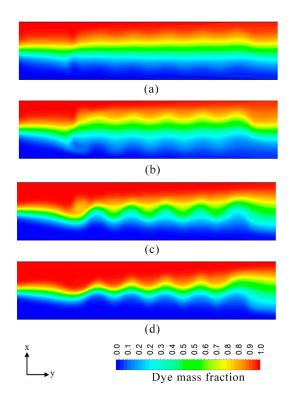
**Figure 14.** Dye mass fraction distributions on *x-y* plane along the channel length at  $z/H_c = 0.5$  for E = 400 V/cm: (a)  $P_w/W_c = 0.2$ ; (b)  $P_w/W_c = 0.43$ ; (c)  $P_w/W_c = 0.5$ ; and (d)  $P_w/W_c = 0.6$ .
