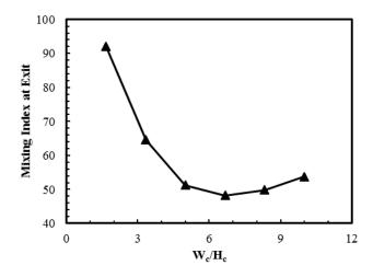
**Figure 9.** Effect of  $W_c/H_c$  on mixing index at the exit.
