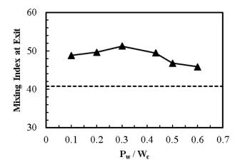
**Figure 13.** Effect of  $P_{\rm W}/W_{\rm c}$  on mixing index at the exit (homogeneous channel, dashed line; heterogeneous channel, solid line with symbols).
