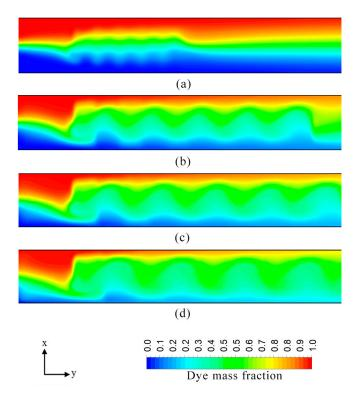
**Figure 12.** Dye mass fraction distributions on *x-y* plane along the channel length at  $z/H_c = 0.5$  for E = 400 V/cm: (a)  $P_L/W_c = 0.2$ ; (b)  $P_L/W_c = 0.43$ ; (c)  $P_L/W_c = 0.5$ ; and (d)  $P_L/W_c = 0.6$ .
