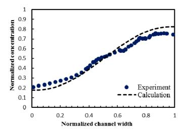
**Figure 5.** Validation of the numerical results for normalized concentration profile across the channel width using experimental data (Wu and Li [18]).
