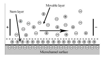
Figure 3. Schematic of electric double layer.
