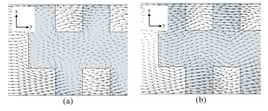
**Figure 7.** Velocity vectors on *x-y* plane: (a)  $z/H_c = 0.2$  and (b)  $z/H_c = 0.45$ .
