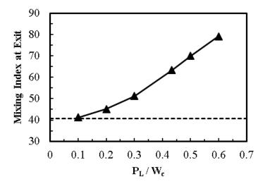
**Figure 11.** Effect of  $P_L/W_c$  on mixing index at the exit (homogeneous channel, dashed line; heterogeneous channel, solid line with symbols).
