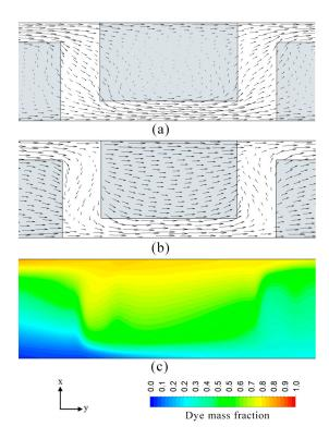
**Figure 16.** Flow and mixing visualization in the proposed micromixer in the *x-y* plane at E = 400 V/cm: (a) velocity vectors in *x-y* plane at  $z/H_c = 0.3$ ; (b) velocity vectors at  $z/H_c = 0.6$ ; and (c) Dye mass fraction distribution in *x-y y-x* at  $z/H_c = 0.5$ .
