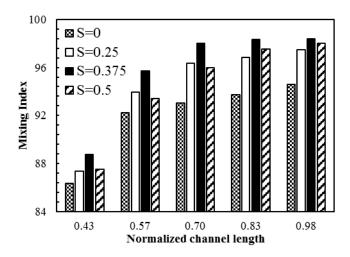
**Figure 17.** Comparison of the mixing index developments along the normalized channel length among the micromixers with different patch spaces at E = 400 V/cm.
