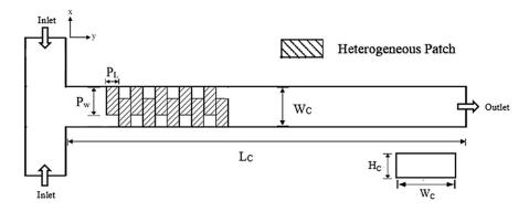
Figure 1. Schematic diagram and geometric parameters.
