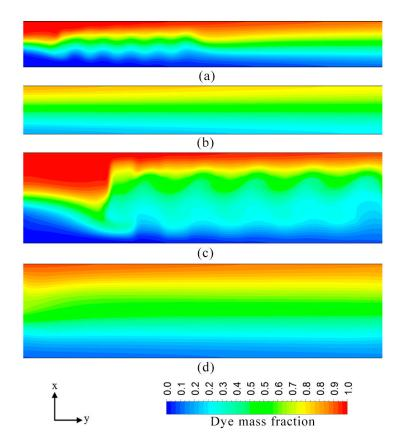
**Figure 10.** Dye mass fraction distributions on *x-y* plane at  $z/H_c = 0.5$  for E = 400 V/cm: (a)  $W_c/H_c = 3.33$ ; near inlet  $(x/L_c = 0.05-0.42)$ ; (b)  $W_c/H_c = 3.33$ ; near exit  $(x/L_c = 0.56-1.0)$ ; (c)  $W_c/H_c = 8.33$ ; near inlet  $(x/L_c = 0.15-0.5)$ ; and (d)  $W_c/H_c = 8.33$ ; near exit  $(x/L_c = 0.6-1.0)$ .
