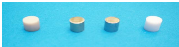
Fig. 2: Tested substrates (from left to right: zirconia ceramic, non-precious gold alloy, nickel-chromium alloy and white substrate)
