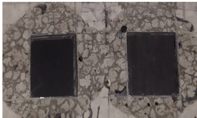
Figure 3. View of the CFRP tape pieces glued to the cleaned surface (ER52 series).
