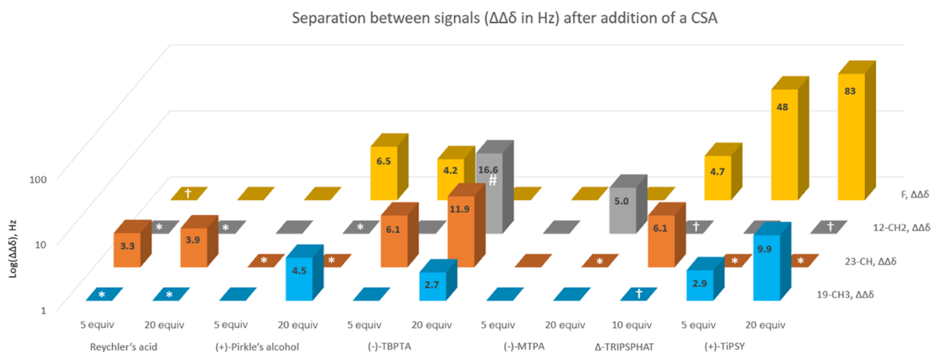
Figure 3. CSA-induced separation of signals in ^1\text{H} and ^{19}\text{F} NMR spectra. The numbers in the bars represent \Delta\Delta\delta in linear scale in Hz. *Resonance obscured by CSA or residual water peaks. †Resonance(s) of MRTX1719 broad. #Only de-shielded doublet observed cleanly.
