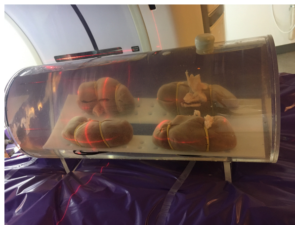
Figure 1. Water-filled phantom with four porcine kidneys attached to a plastic ledge. The mean circumference for an average 9 years old boy/girl: 63.6cm/62.6cm respectively while the phantom circumference is 63cm.
