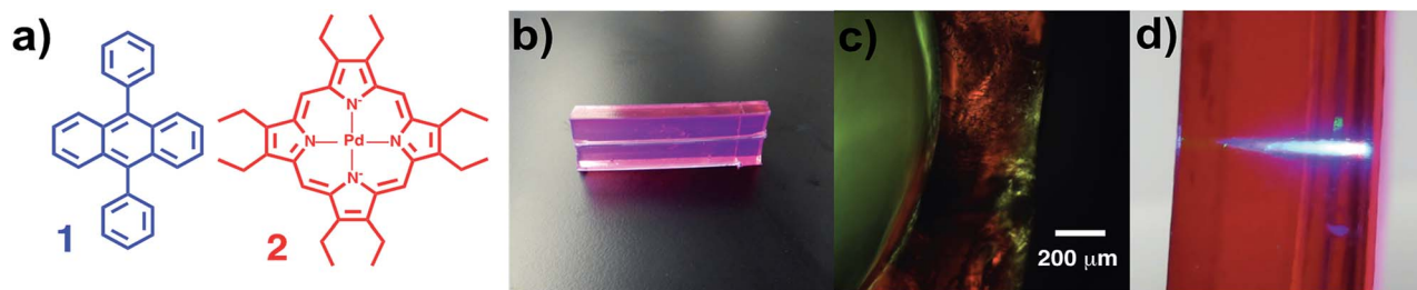
Fig. 2 (a) Dye-sensitizer pair for upconversion of greenlight to blue light, dye: diphenylanthracene (1), sensitizer: 2,3,7,8,12,13,17,18-octaethyl-21H,23H-porphine palladium(II) (2); (b) microreactor demonstrating upconversion enrichment of blue photon flux in diffuse sunlight; (c) cross-section of reactor surface showing depth of coating on channel; (d) dye-doped reactor upconverting a 532 nm (green) laser.
