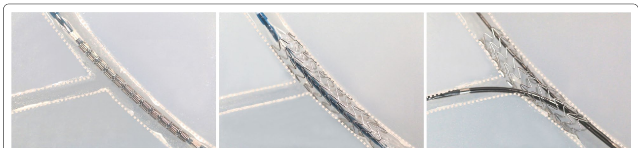
Fig. 3 Side-branch expansion in the in vitro experiment using a phantom bifurcation model
