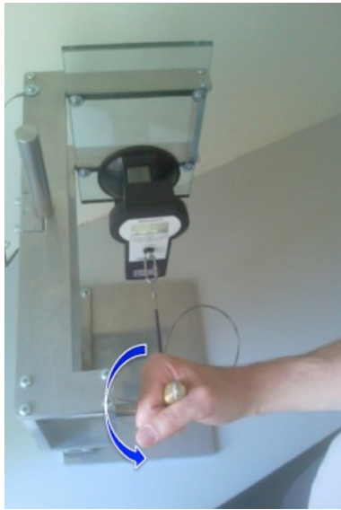
Fig. 2 Setup for pronation strength measurement: the blue arrow indicates the isometric pronation directional movement
