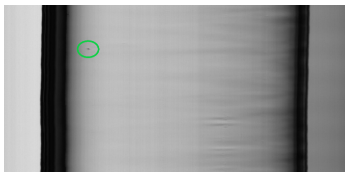
Figure 4. A blob defect (enclosed in a green oval). The tube has a more similar shape to a “sausage”, as can be seen on the center and right side.
