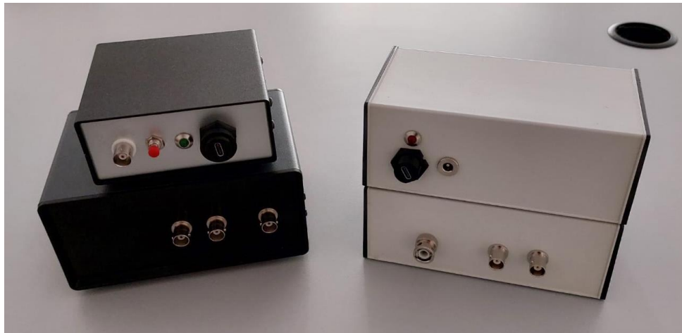
Figure 2 - A few examples of how the circuit can be arranged into a case. Note that their design can be different, since you can flexibly add features according to your needs.
