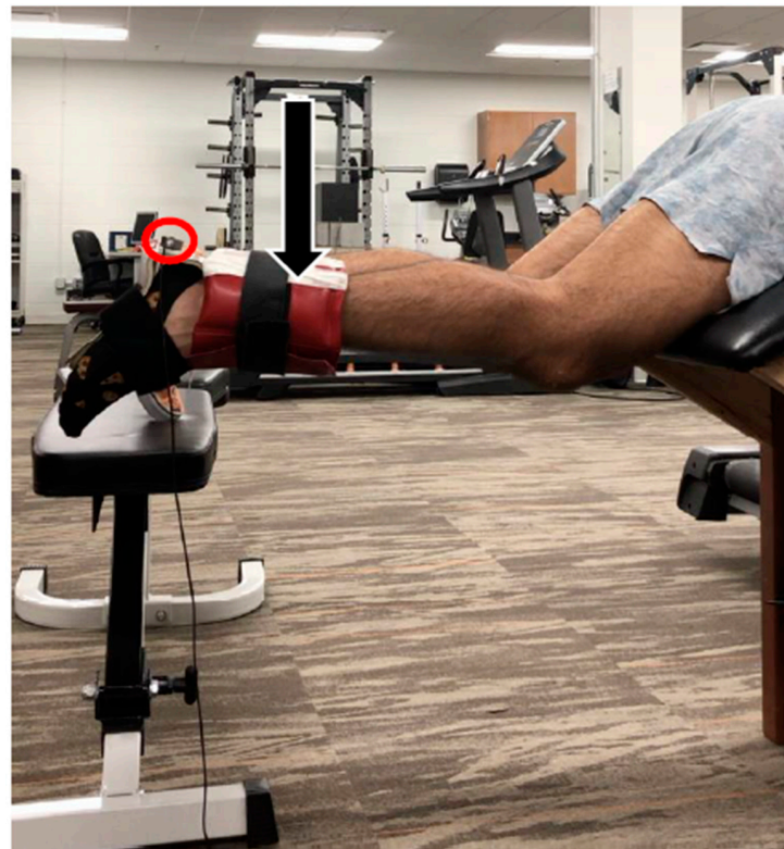
Figure 1. Experimental setup for assessment of active hamstring muscle-tendon stiffness. Subjects were fitted with a rigid ankle splint, a load corresponding to 25% MVIC, and a tri-axial accelerometer (circled in red). A member of the research team applied a downward manual perturbation (indicated by the downward black arrow) to obtain the damped oscillation which was viewed and analyzed offline.
