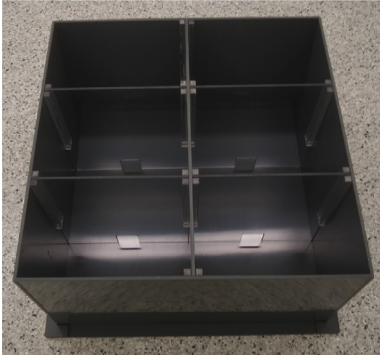
Fig. 8. Dimensions, in cm, for the custom construction of a modular testing apparatus (A). A modular design allows for diverse uses: a single large open field arena, multiple smaller open field arenas of various sizes, or 2 two- or three-chamber arenas (mice: B , rats: C ), and facilities easy cleaning of the dividers, partition, and base (D, exterior of apparatus lifted off base during cleaning).
