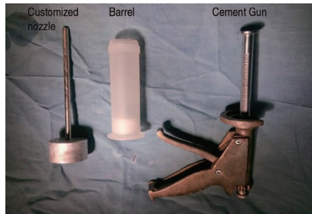
Fig. 2. Cementing apparatus comprised of barrel, nozzle and the cement gun.
