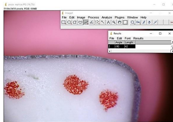
Figure 4. Replica technique with silicon in ImageJ.
