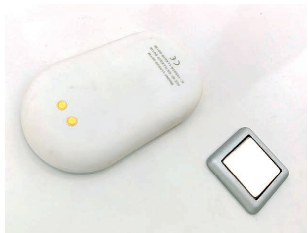
Fig. 1. The posture-correcting device (LumoLift) consisted of an accelerometer and a magnet, calibrated in neutral position.
