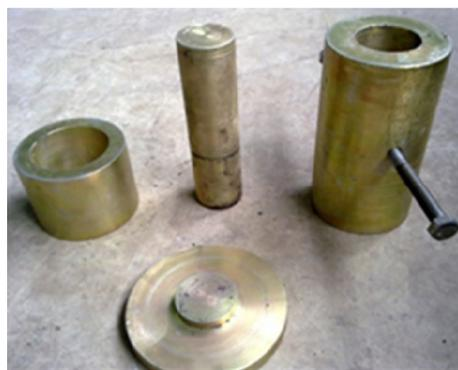
**Figure 2.**  $\Phi 50\text{mm} \times 100\text{ mm}$  pressing mold.
