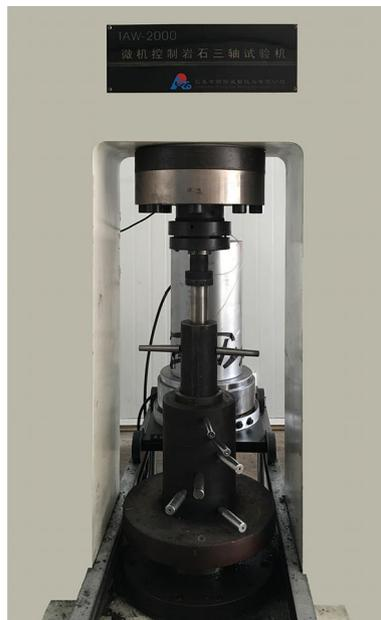
**Figure 1.** Rock triaxial testing machine controlled by TAW-2000 microcomputer.
