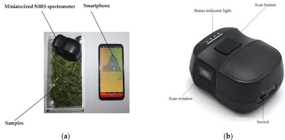
Figure 2. Miniaturized NIRS system, (a) spectrum acquisition process, and (b) miniaturized NIRS spectrometer [25]. For spectrum acquisition, the scan window of the miniaturized NIRS spectrometer is placed close to the samples and the scan button is then pressed, and the acquired spectrum is displayed on the smartphone.
