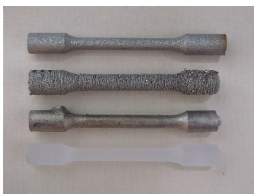
Figure 3. Exterior appearance of (a) an LBM specimen; (b) an EBM specimen; (c) a cast Ti-6Al-4VELI specimen; and (d) a plastic dumbbell pattern.
