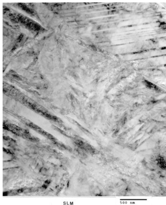
Figure 12. TEM view of SLM \alpha - \alpha' martensite and twinned \alpha .
