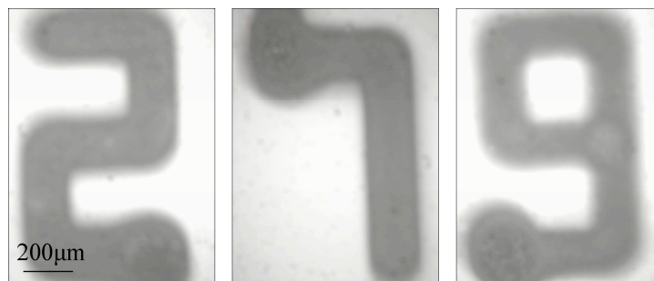
Figure 7. Optical images of Arabic number '2', '7', and '9'. The applied voltage, the flow rate of solution, the velocity of substrate, the distance between nozzle and collector and the deposition time were 1.5 kV, 50 \mu L/h, 5 mm/s, 5 mm, and 15 s, respectively.
