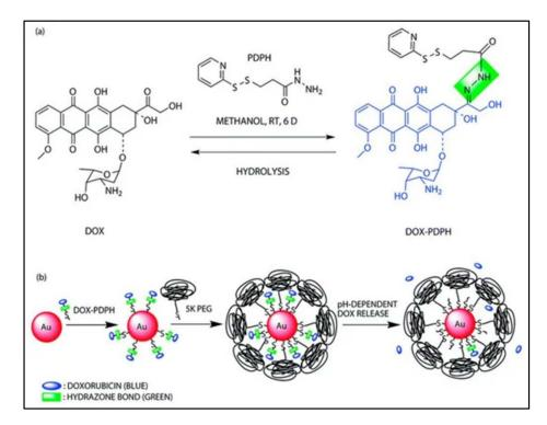
**Figure 11.** A pH-sensitive drug-gold nanoparticle system: (a) chemical synthesis of the doxorubicin-hydrazone linker conjugate (dox–PDPH); (b) schematic illustration of the synthesis of the multifunctional drug delivery system and its pH-dependent doxorubicin release [82].
