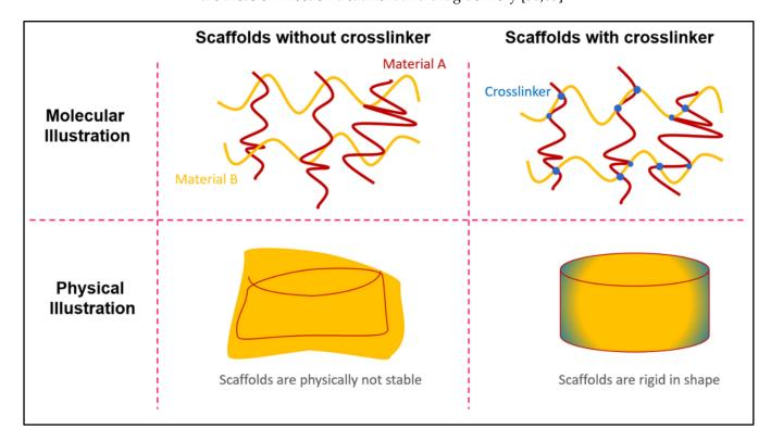
Figure 5. Illustration of the enhancement of a scaffold's mechanical properties by employing the crosslinking processes.
