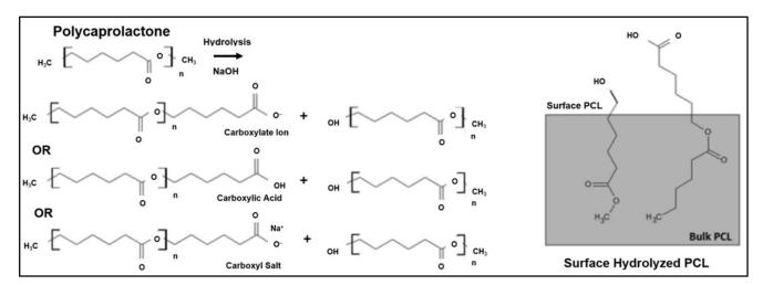
Figure 8. The hydrolytic degradation mechanism of PCL scaffolds [79].
