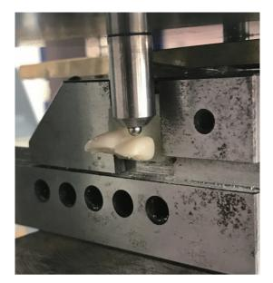
**Fig. 2.** Point of application of the shear forces and illustration of the device.
