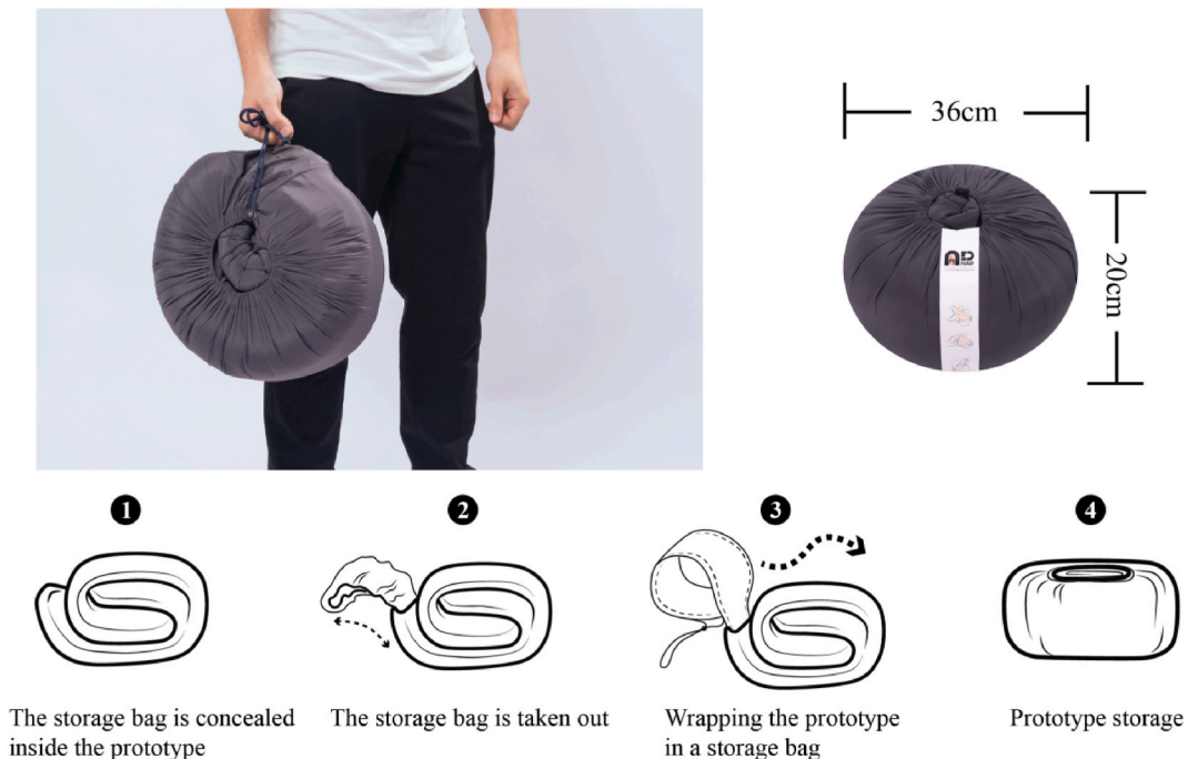
Fig. 3. Schematic diagram of the storage function of the prototype.
