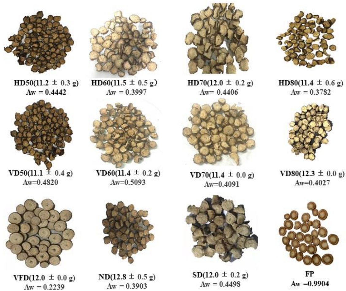
Figure 1. Appearance and dry weight of dried burdock root treated by different drying methods. ( n = 3 ; the fresh weight for burdock is 60 g, and the dry weight are expressed as Mean \pm SD; HD50–80 means hot air drying at 50–80 °C, VD50–80 means vacuum drying at 50–80 °C, VFD means vacuum freeze drying, ND means natural drying, SD means sun light drying, FP means fresh pieces and Aw means activity water).
