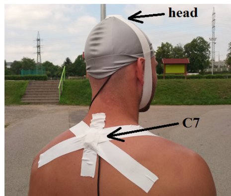
Figure 4. Acceleration sensor placed on the test subject's head and C7 vertebrae.
