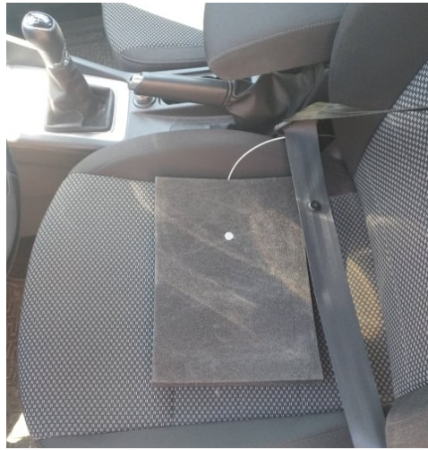
Figure 3. Acceleration sensor placed on the seat of the vehicle under the driver's buttock.
