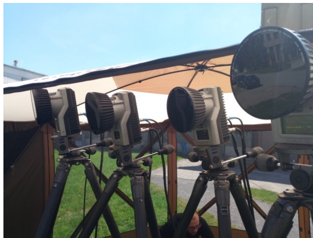
Figure 5. Device for measuring the exact speed of the vehicle—System Qualisys.
