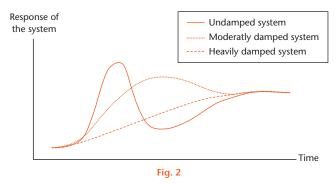
Graph showing the response of differently damped systems to 'response of the system'. The solid line represents an undamped system, the dotted line a moderately damped system and the dashed line, a heavily damped system. In clinical practice, it has been suggested that the uptake of agents such as platelet rich plasma follow the solid line, whereas others such as metal-on-metal hip arthroplasties follow the dotted line, and vitamin C uptake the dashed line.
